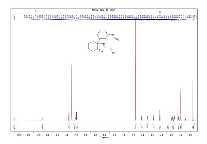
**Lab Notes:** The sample contained the highly pure compound MXiPR in its HCl salt form with barely any <sup>1</sup>H NMR active impurities.
